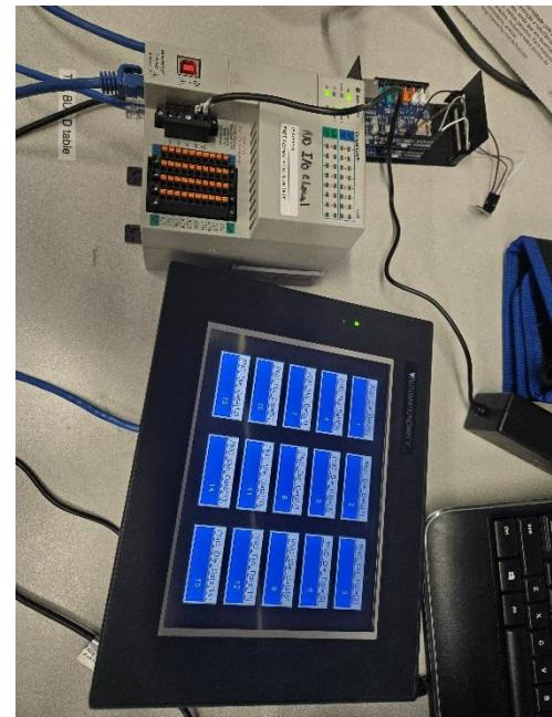
publication documents exactly how to configure this. Marc Kramer was able to help me with this by showing data exchange between Raspberry PI and an Allen Bradley PLC. In the end though we used Modbus for communication because there was no library that could handle ethernet/ip for Arduino and doing ethernet over IP without a library was also very hard and involved a lot of memory management techniques that I could not wrap my head around fully.
