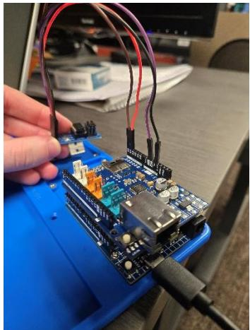
This is the Die Ignition project that I helped with as an intern at Pridgeon and Clay. In this project we needed a reliable method to automatically detect and record when tooling or a press die is loaded into a machine, along with the identity of the die set being used. We had to find a way to capture this information onto an Arduino Uno R4 Minima.
